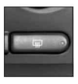
If the vehicle has heated mirrors, the button to turn this function on or off is located on the climate control panel.
